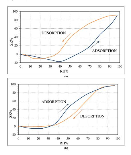
Figure 10. Sensor response towards relative humidity of (a) OSR700; (b) SWP700 biochars.
