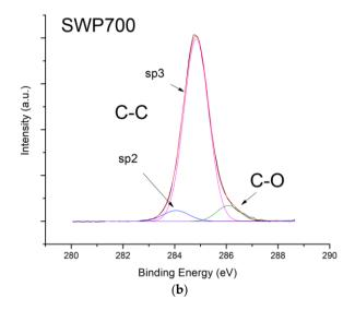
**Figure 4.** High resolution X-ray photoelectron spectroscopy (XPS) spectra of C1s peak for **(a)** OSR700; **(b)** SWP700.
