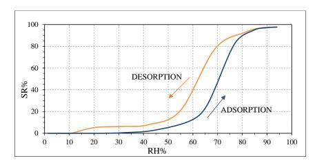
Figure 11. Polyvinylpyrrolidone (PVP) sensor response toward relative humidity.
