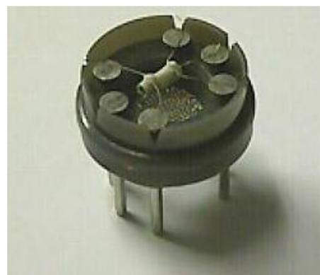
**Figure 1.** Schematization and picture of Taguchi chemoresistive gas sensor.
