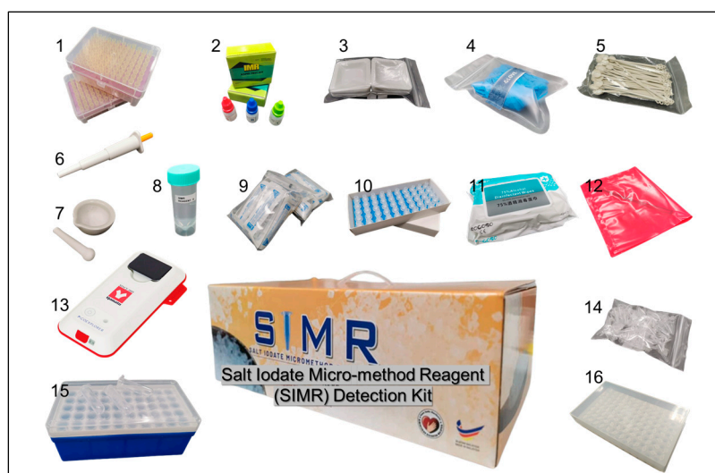
Figure 1. Overall illustration of SIMR detection kit, containing the complete content for on-site analysis, including: (1) pipet tips; (2) IMR iodine RTK-containing solution A, B, and C; (3) weighing boats; (4) Nitrile gloves; (5) plastic spatula; (6) mini pipet; (7) pestle and mortar; (8) SIMR reagent A; (9) 3 mL syringe; (10) 13 mm nylon filter (0.45 µm pore size); (11) 75% alcohol wipe; (12) disposal bag with zip tie; (13) portable photo absorbance reader; (14) 0.2 mL tubes for sample scooping; (15) rack with 5 mL sample tube containing pre-filled 4 mL of deionized water; and (16) 0.2 mL tube rack pre-filled with SIMR reagent B.
