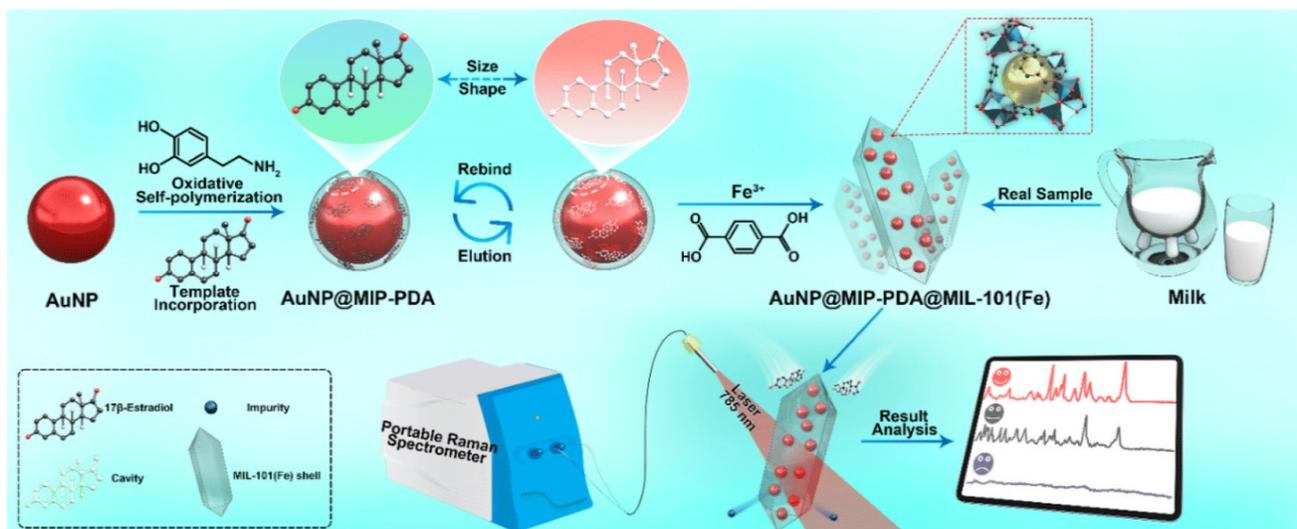
**Figure 8.** Schematic of torpedo-shaped MOFs wherein E2-molecule-imprinted polymer-coated AuNPs are anchored (AuNP@MIP-PDA@MIL-101(Fe)) for SERS-based detection of E2. The MOF is MIL-101. (MIP: molecularly imprinted polymer, PDA: polydopamine.) Used with permission of the Royal Society of Chemistry, from Ref. [37]; permission conveyed through Copyright Clearance Center, Inc.
