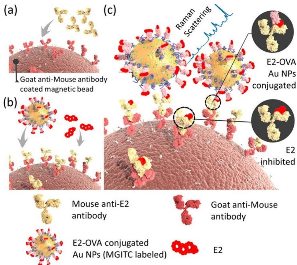
**Figure 6.** Schematic showing the E2 detection with the SERS nanotags. (a) Binding a primary antibody (yellow) with a secondary antibody (red) pre-immobilized on a magnetic bead; (b) competitive immunoreaction between E2 molecules and a AuNP-based SERS nanotag; (c) post-immunoreaction step before SERS measurement. (E2, 17 $\beta$ -estradiol; OVA, ovalbumin; MGITC, malachite green isothiocyanate.) Reprinted with permission from Ref. [35]. Copyright 2016 American Chemical Society.
