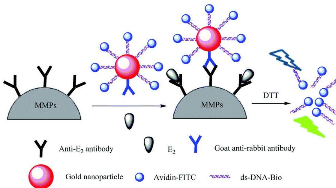
**Figure 2.** Schematic showing a fluorescence-based competitive immunoassay for E2. (MMP; magnetic microparticles, DTT; dithiothreitol.) Used with permission of the Royal Society of Chemistry, from Ref. [29]; permission conveyed through Copyright Clearance Center, Inc.
