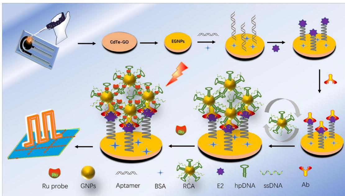
**Figure 11.** Schematic showing the working principle of the photoelectrochemical aptasensor (CdTe, cadmium telluride quantum dots; GO, graphene oxide; EG-NP, electrodeposited gold nanoparticle; BSA, bovine serum albumin; E2, 17 $\beta$ -estradiol; RCA, rolling circle amplification; hpDNA, hairpin DNA; ssDNA, single-stranded DNA; Ab, antibody). Reprinted from Ref. [58], Copyright 2022, with permission from Elsevier.
