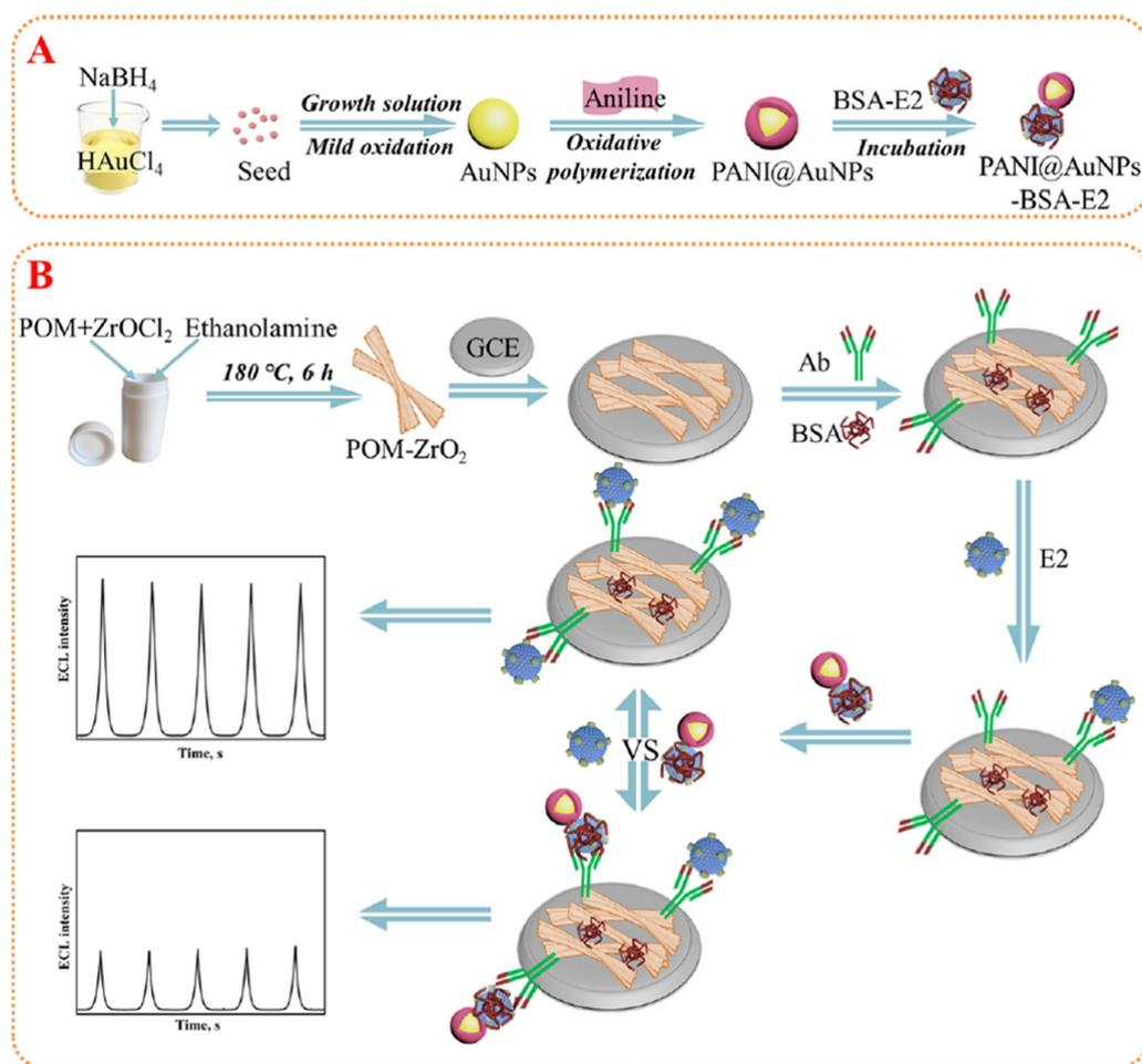
**Figure 3.** Schematic showing the dual-quenching-based competitive immunoassay in electrochemiluminescence (PANI, polyaniline; AuNPs, Au nanoparticles; POM, polyoxomolybdate; GCE, glassy
