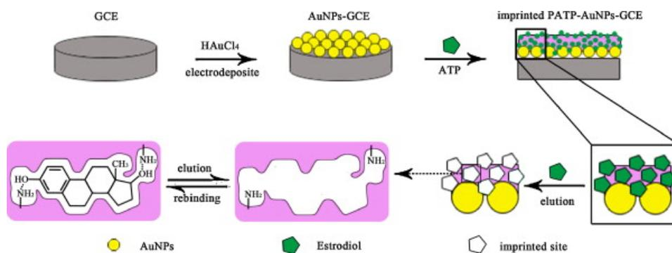
**Figure 4.** Fabrication process of an MIP-modified electrode. (GCE, glassy carbon electrode; AuNPs, Au nanoparticles; ATP, p-aminothiophenol.) Reprinted from Ref. [46], Copyright (2014), with permission from Elsevier.
