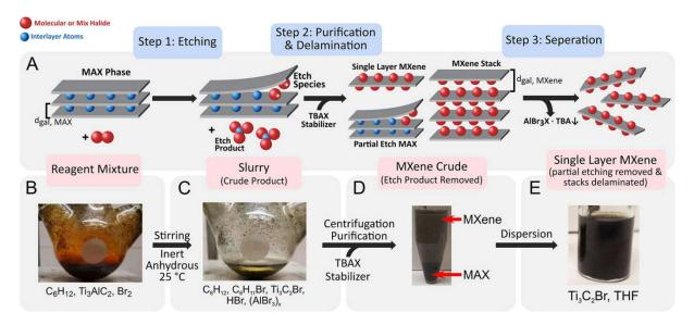
**Figure 2.** (A–E) Halogen etching procedure of the MAX phase. Tetrahydrofuran was used as the stable colloidal solution. Reprinted and adapted with permission from [64]. Copyright 2021 American Chemical Society.
