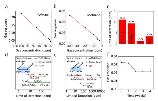
Figure 8. (a–f) Gas response variation of monolayer  $V_2CT_x$  MXene flakes to different types of gases. Reprinted and adapted with permission from [123]. Copyright 2019 American Chemical Society.
