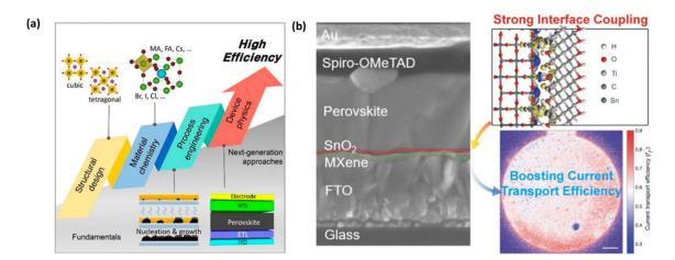
**Figure 16.** (a) Perovskite solar cell, (b) Interface boosting charge transport. Reprinted and adapted with permission from [156,159]. Copyright 2020 American Chemical Society.
