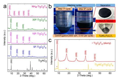
**Figure 4.** ( $\mathbf{a}$ – $\mathbf{c}$ ) XRD results of  $\mathrm{Ti}_3\mathrm{C}_2\mathrm{T}_{\mathrm{X}}$  MXene prepared with different concentrations of HF solution. Reprinted and adapted with permission from [5]. Copyright 2017 American Chemical Society.
