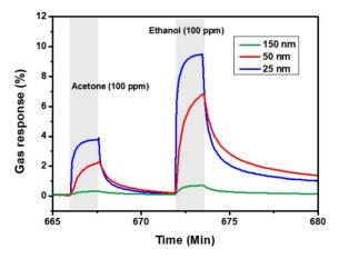
**Figure 6.** Thickness-dependent responses of  $Ti_3C_2T_x$  MXene to various gases at a fixed concentration of 100 ppm. Reprinted and adapted with permission from [32].
