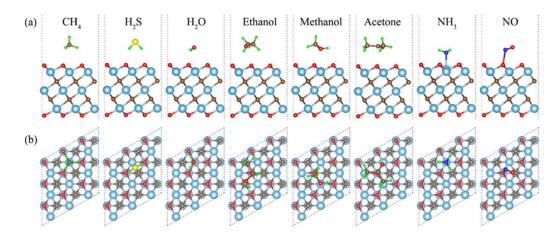
Figure 7. (a,b) Side and top views of the optimized structure of eight gas molecules adsorbed on  $Ti_3C_2T_x$  MXene. Reprinted and adapted with permission from [22]. Copyright 2019 American Chemical Society.
