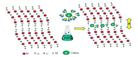
**Figure 3.** Schematic of an increase in the d-spacing of  $Ti_3C_2T_x$  MXene with intercalation using cations. Reprinted and adapted with permission from [70].
