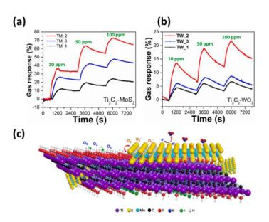
**Figure 9.** (a,b) Comparison of the response behaviors of  $MoS_2/Ti_3C_2T_x$  and  $WO_3/Ti_3C_2T_x$  composites to  $NO_2$  gas. (c)  $NO_2$ -sensing mechanism of  $MoS_2/Ti_3C_2T_x$  composite. Reprinted and adapted with permission from [125].
