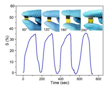
**Figure 10.** Gas-sensing signal of the as-prepared PEDOT:PSS/ $Ti_3C_2T_x$  composite to 100 ppm NH<sub>3</sub> gas at a variety of bending angles (60°, 120°, 180°, 240°). Reprinted and adapted with permission from [109]. Copyright 2020 American Chemical Society.
