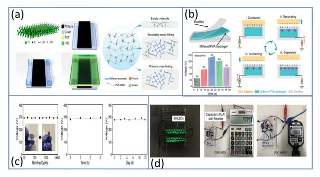
**Figure 13.** (a) Structure of  $Ti_3C_2T_x$  MXene and MXene triboelectric nanogenerator (MXene TENG) assembled as shown in the schematics. (b) MXene/PVA hydrogel flexible multifunctional TENG. (c) Mechanical stability and reliability of EAPs-based TENG with diverse applications. (d) The 50 LEDs, calculator, and stopwatch were powered by the TENG. Reprinted and adapted with permission from [139,142–144].
