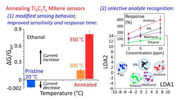
**Figure 11.** VOC-sensing activity of oxidized TiO<sub>2</sub>/Ti<sub>3</sub>C<sub>2</sub>T<sub>x</sub> composite. Reprinted and adapted with permission from [132]. Copyright 2020 American Chemical Society.
