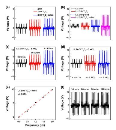
**Figure 14.** (a–f) Output performance of PENG fabricated with Li:ZnO/Ti<sub>3</sub>C<sub>2</sub>T<sub>x</sub> composites. Reprinted and adapted with permission from [147]. Copyright 2022 American Chemical Society.
