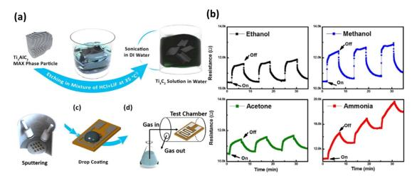
**Figure 5.** ( $\mathbf{a}$ , $\mathbf{c}$ , $\mathbf{d}$ ) Schematic of the  $\mathrm{Ti}_3\mathrm{C}_2\mathrm{T}_{\mathrm{X}}$  gas-sensing material and ( $\mathbf{b}$ ) its sensing signals of various toxic gases of 100 ppm at room temperature. Reprinted and adapted with permission from [118]. Copyright 2017 American Chemical Society.
