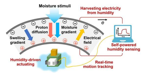
**Figure 15.** MXene for harvesting energy with moisture stimuli. Reprinted and adapted with permission from [155]. Copyright 2021 American Chemical Society.
