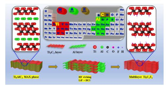
**Figure 1.** Schematic of Ti<sub>3</sub>C<sub>2</sub>T<sub>x</sub> MXene preparation from the Ti<sub>3</sub>AlC<sub>2</sub> MAX phase. Reprinted and adapted with permission from [11]. Copyright 2021, Elsevier.
