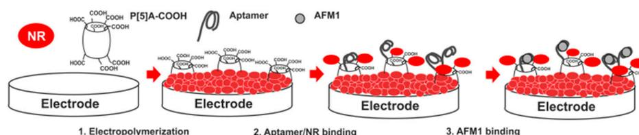
**Figure 14.** The scheme of an aflatoxin M1 aptasensor based on electropolymerized neutral red (NR) at presence of pillar[5]arene (P[5]A-COOH). The  $NH_2$ -modified DNA aptamers specific to aflatoxin M1 (AFM1) were covalently attached to the carboxylic group of P[5]A-COOH activated by carbodiimide chemistry. Adopted from [79] with the permission of Wiley-VCH.
