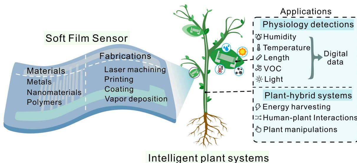
**Figure 1.** Overview of micro/nano soft film sensors for the establishment of intelligent plant systems.
