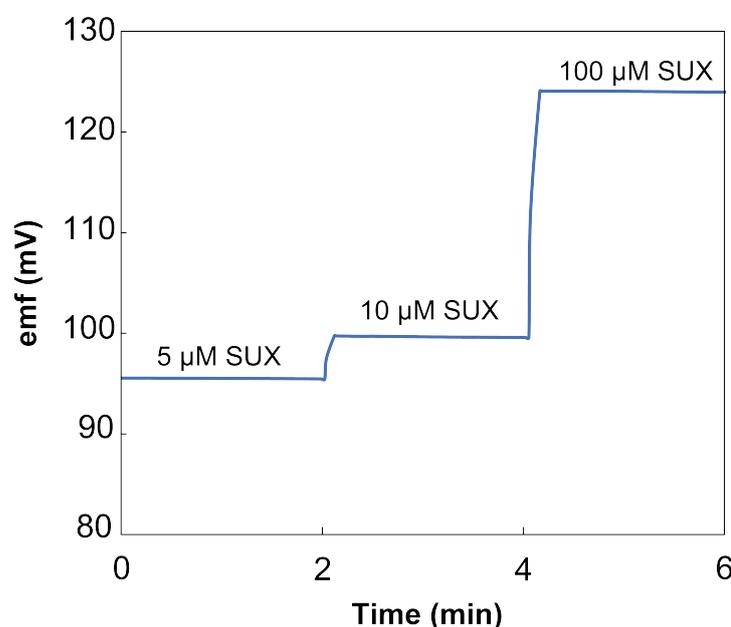
**Figure 5.** The *emf* traces from recovery experiments where thread-based ISEs were exposed to 5, 10, and 100  $\mu\text{M}$  concentrations of SUX in 20% urine.
