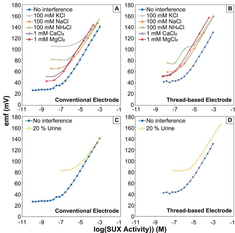
**Figure 3.** The response curves for (A,C) conventional ISEs and (B,D) the thread-based ISEs in the presence of a fixed concentration of interfering cations. (A,B) The interfering inorganic salts caused LODs to increase in both conventional ISE and thread-based ISE systems. (C,D) Unknown urine content caused larger increases in LOD in both systems.
