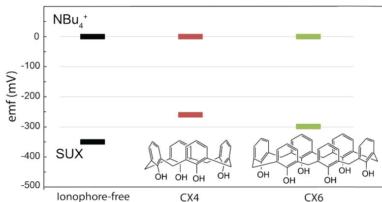
**Figure 4.** The differences in the *emf* of the SUX ISE for 10 mM SUX solution with respect to 10 mM  $\text{Bu}_4\text{N}^+$  (black trace shows an ionophore-free sensing membrane, red trace shows the CX4 ionophore in the sensing membrane, and the green trace shows the CX6 ionophore in the sensing membrane).
