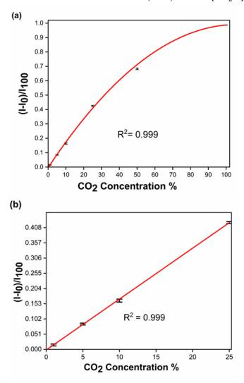
**Figure 6.** Variation of  $(I - I_0)/I_{100}$  with CO<sub>2</sub> concentration in N<sub>2</sub> of (**a**) 0–100% (entire range, polynomial fit) and (**b**) 0–25% (linear range).
