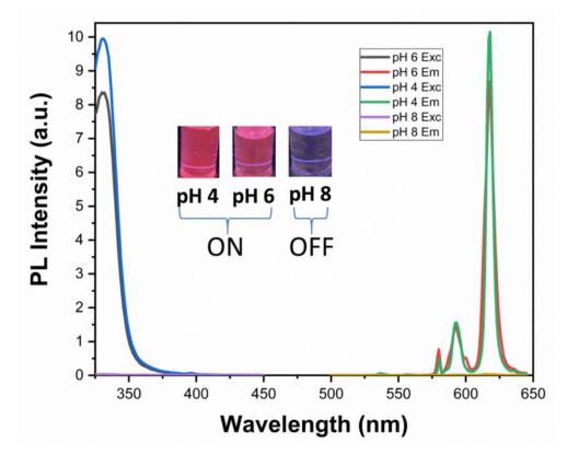
**Figure 2.** Photoluminescence spectra of K[Eu(hfa)<sub>4</sub>] in solution at pH 4, 6, and 8. Right traces ( $\lambda > 500 \text{ nm}$ ) show emission spectra dominated by the sharp  ${}^5D_0 \rightarrow {}^7F_J$  atomic Eu(III) emission lines, while left traces ( $\lambda < 450 \text{ nm}$ ) show excitation spectra dominated by the broad hfa ligand-based transitions. Inset shows emission pictures under UV light irradiation at respective pH values.
