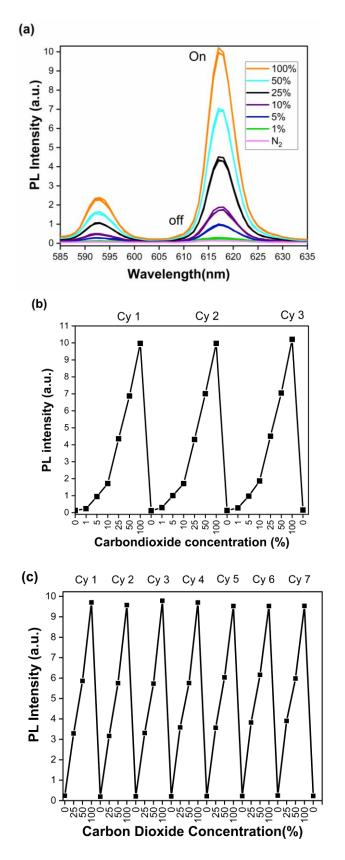
**Figure 5.** (a) PL spectra of the sensor after exposure to 1%, 5%, 10%, 25%, 50%, and 100% of CO<sub>2</sub> in N<sub>2</sub>. (b) PL peak intensity changes for three purging cycles using 1%, 5%, 10%, 25%, 50%, and 100% of CO<sub>2</sub> in N<sub>2</sub>. (c) PL peak intensity changes for seven purging cycles using 25%, 50%, and 100% of CO<sub>2</sub> in N<sub>2</sub>.
