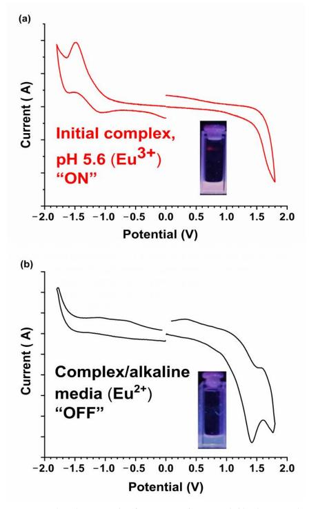
**Figure 3.** Cyclic voltammetry data for 1 at 0.5 mg/0.5 mL in dichlorobenzene solvent and TBAClO<sub>4</sub> electrolyte (**a**) at pH 5.6 and (**b**) at pH 8.0. The inset pictures show the complex under a UV lamp at the respective pHs.
