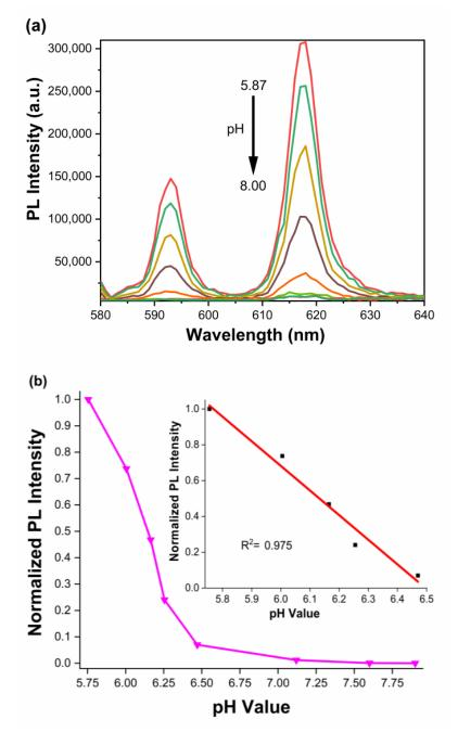
**Figure 4.** (a) PL spectra of  $K[Eu(hfa)_4]$  with different pH values from pH 5.87 to pH 8.0. (b) PL titration at 618 nm at different pH, the inset shows the linear relationship from pH 8.8 to 6.5 with  $R^2$  of 0.975.
