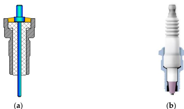
**Figure 1.** Ion probe design in the form of a (a) needle and (b) spark plug.
