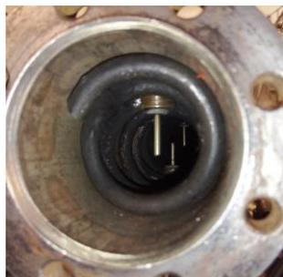
**Figure 12.** The internal view on the tube section with a Shchelkin spiral and ion sensors mounted between spiral turns.
