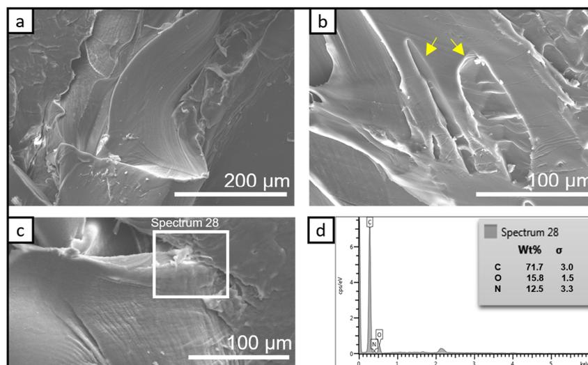
**Figure 1.** Representative SEM micrographs of bio-PA1010, reference sample: low magnification image showing the smooth surface and the demoulded area of the sample (a); detailed image of the technological cavities (marked in b) with yellow arrows); the area selected for the EDS analysis (c); and the EDS spectrum and elemental composition of the selected area (d).
