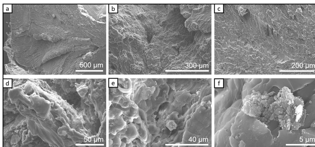
**Figure 5.** Representative SEM micrographs of bio-PA1010 filled with 4% C500 graphene nanoplatelets after thermal treatment at 80 °C (a); low magnification images of the sample with progressive magnification showing the smooth surface and embedded graphenic aggregates (b–f).
