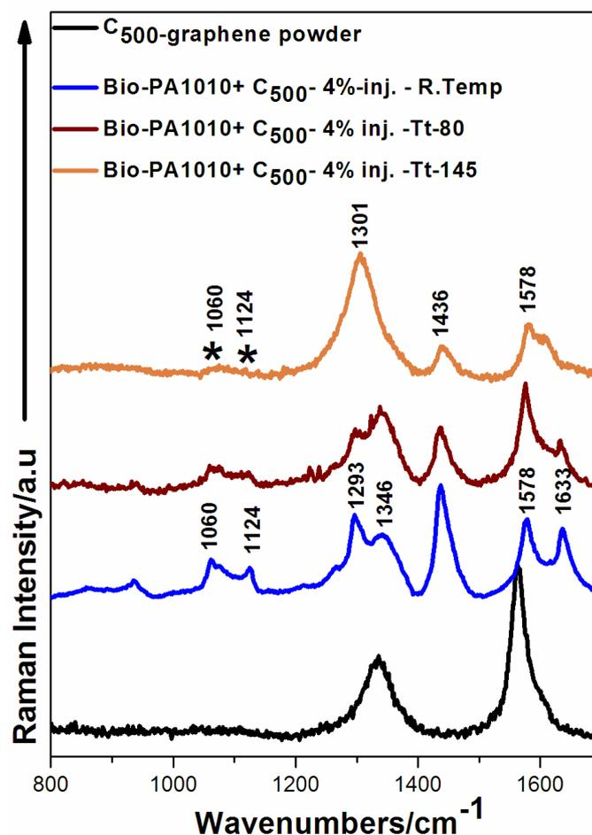
**Figure 10.** The Raman spectra of bio-PA1010 nanocomposite filled with GNP C500-4% thermally treated at 80 °C and 145 °C. We marked with \* the bands that are less visible after the thermal treatment.
