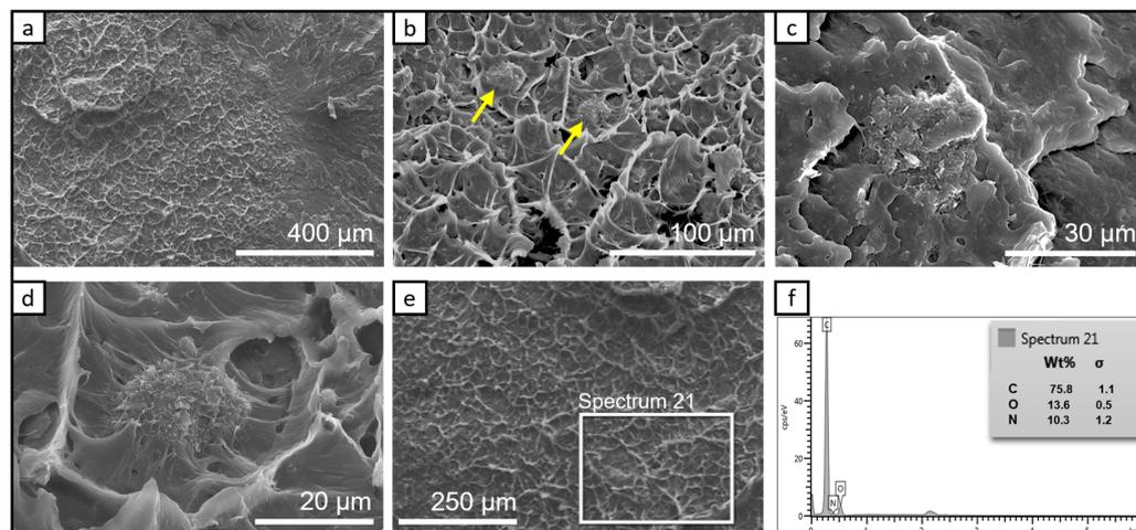
**Figure 3.** Representative SEM micrographs of bio-PA1010 filled with 4% C500 GNP: low magnification image showing the rough surface of the sample (a); detailed view of the rough surface, with flakes and graphenic aggregates marked with yellow arrows (b,c); and high magnification image of graphenic aggregates surrounded by flakes (d); the area selected for the EDS analysis (e); and the EDS spectrum and elemental composition of the selected area (f).
