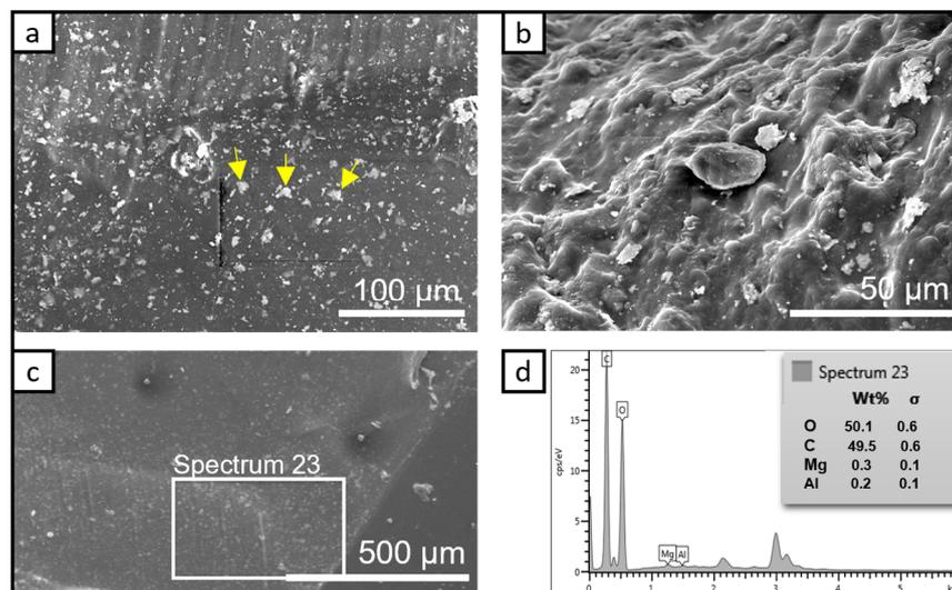
**Figure 2.** Representative SEM micrographs of bio-PA1010 nanocomposites filled with LDH 5%: low magnification image showing the rough surface of the sample, with LDH aggregates (marked in (a) with yellow arrows); detailed view of the LDH aggregates (b); the area selected for the EDS analysis (c); and the EDS spectrum and elemental composition of the selected area (d).
