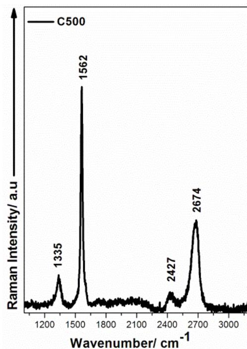
**Figure 9.** The Raman spectra of C500 graphene fillers in the bio-PA1010 samples. Excitation laser: 532 nm.
