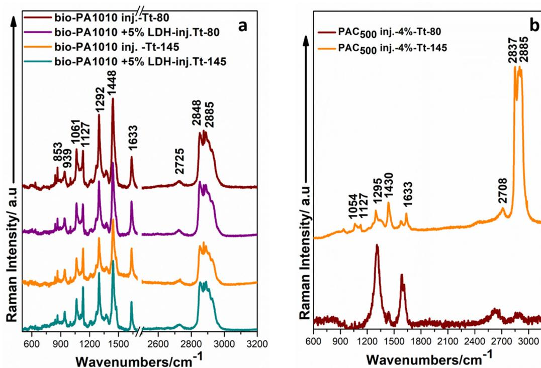
**Figure 11.** Raman spectra of neat bio-PA1010 and filled with LDH, thermally treated at 80 °C and 145 °C, measured after 1 month (a) and of bio-PA1010 nanocomposite filled with graphene type C500-4% thermally treated at 80 °C and 145 °C, measured after 1 month (b).
