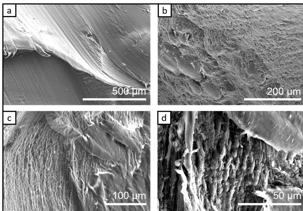
**Figure 4.** Representative SEM micrographs of bio-PA1010 filled with 5% LDH nanocomposites after thermal treatment at 80 °C (a) and low magnification images showing the relatively smooth surface of the sample and detailed views of the small protuberances (b–d).
