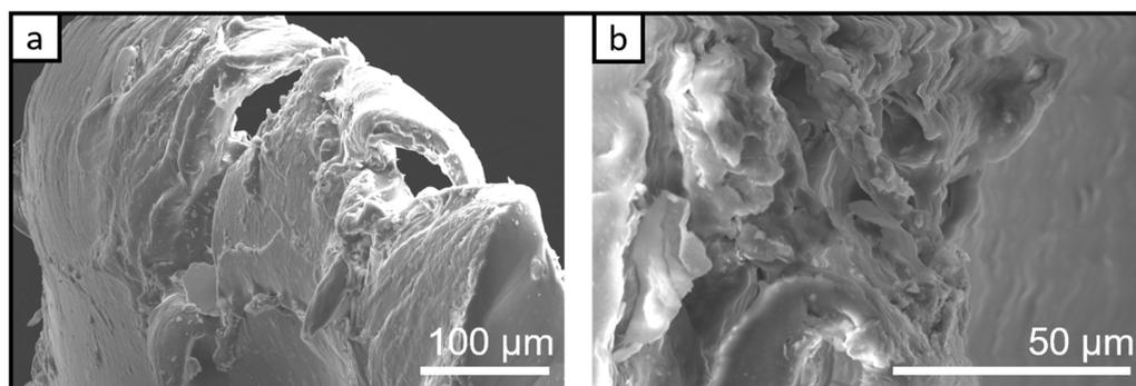
**Figure 6.** Representative SEM micrographs of bio-PA1010 filled with LDH-5% nanocomposites after thermal treatment at 145 °C (a) and low magnification image showing the smooth surface of the sample detailed view of the plastic deformation that occurred in the sample (b).
