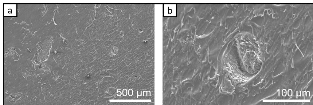
**Figure 7.** Representative SEM micrographs of bio-PA1010 filled with C500-4% nanocomposites after thermal treatment at 145 °C (a,b).
