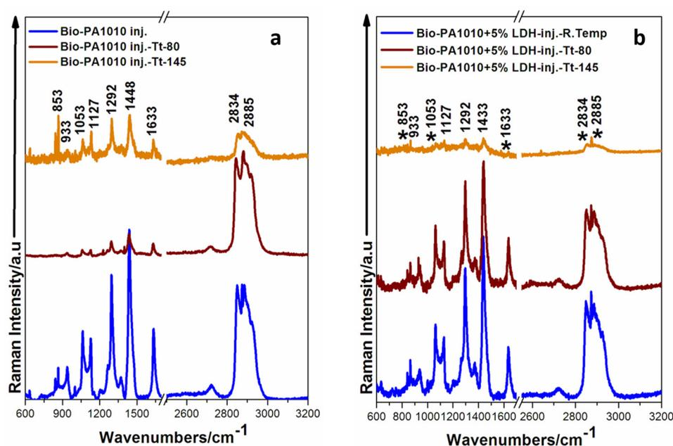
**Figure 8.** The Raman spectra of bio-PA1010 untreated and thermally treated at  $80\text{ }^\circ\text{C}$  and  $145\text{ }^\circ\text{C}$  (a) and bio-PA1010 filled with LDH-5% nanocomposites untreated and thermally treated at  $80\text{ }^\circ\text{C}$  and  $145\text{ }^\circ\text{C}$  (b). We marked with \* the bands that are less visible after the thermal treatment.
