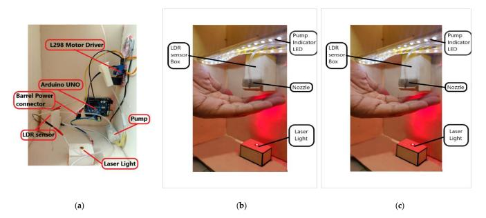
**Figure 3.** Original image of the proposed automated hand sanitizer dispenser; (**a**) placement of Arduino UNO, motor driver and pump, (**b**) setup of laser light, indicator LED, LDR sensor cabinet and nozzle, (**c**) sanitizer dispenser isometric view.
