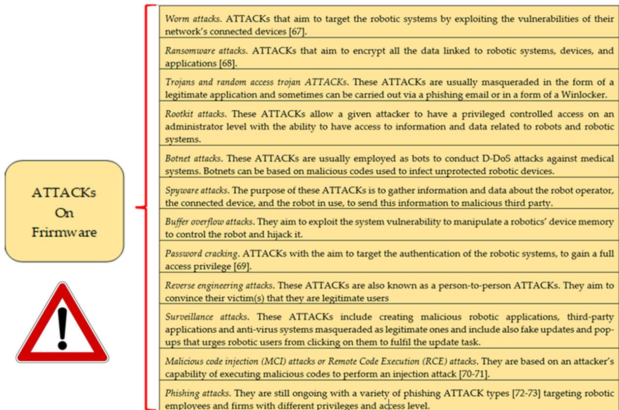
**Figure 3.** Examples of ATTACKs on the firmware.
