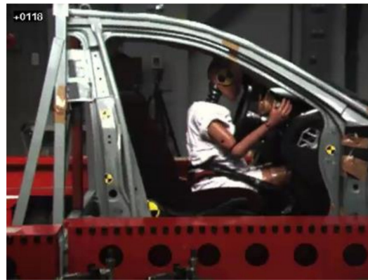
Figure 2. Instant at which the chest of the dummy made contact with the center of the steering wheel in test 1.
