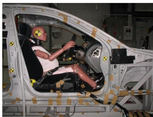
Figure 1. MAMA-2B AF05 ver. sitting in the test setup.
