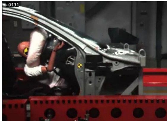
Figure 5. Instant at which the entire dummy's torso slid under the instrument panel in test 3.
