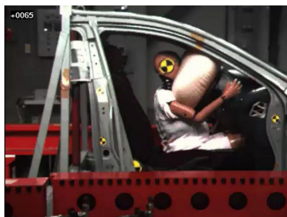
Figure 4. Instant at which the chest of the dummy made contact with the lower rim of the steering wheel in test 2.
