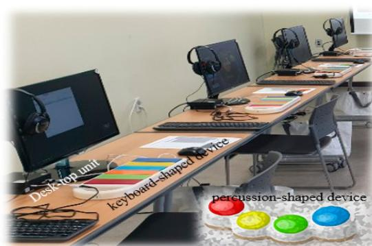
**Figure 2.** Basic settings of devices. Therapeutic musical devices comprise a desk-top unit, monitor, speaker, headphone, and percussion- and keyboard-shaped electrical devices on the desk.
