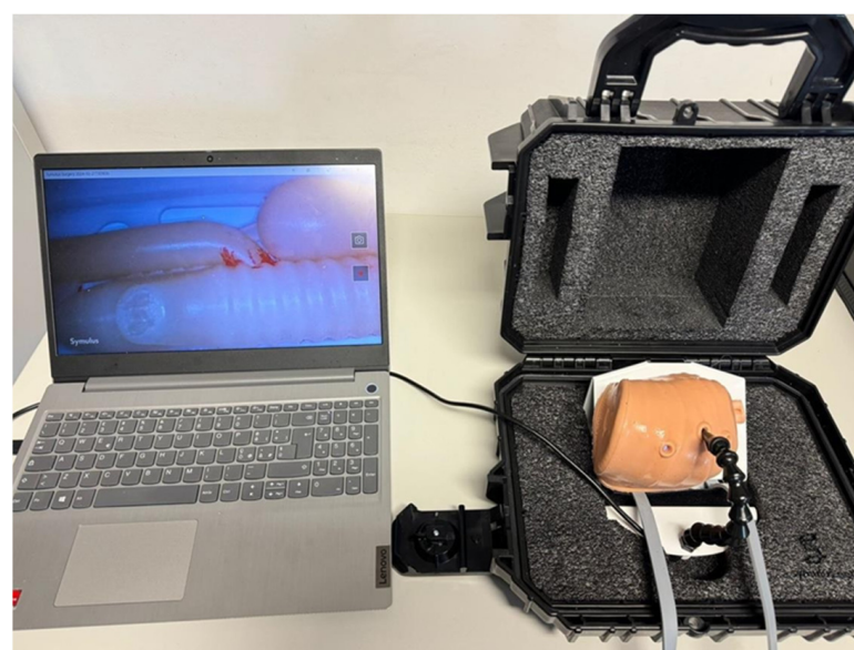
Figure 2. Trainer box with 3D neonatal chest connected to computer screen for the visualization of thoroscopic images.
