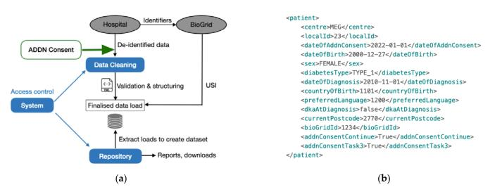
**Figure 6.** (a) Architecture of ADDN registry and data pipelines [12]. (b) An example of patient data with a merged opt-in consent result.
