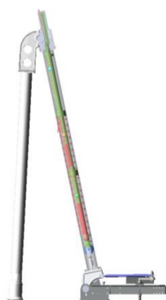
Figure 7. Solid model of GW17 disconnecter.
