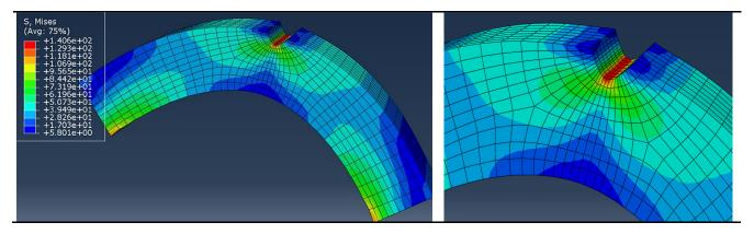
Figure 6. Distributions of Von Mises stress near the notch.
