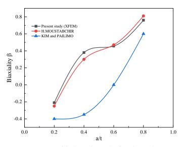
Figure 7. Variation of the biaxiality with a/t at the notch.
