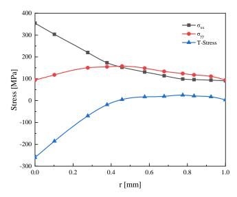
Figure 5. T-stress by stress different method.
