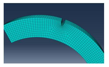
quadratic element C3D20 in the mesh Figure 3, with a size of 0.5 mm. The number of elements is 246117. The number of nodes is 363256.
