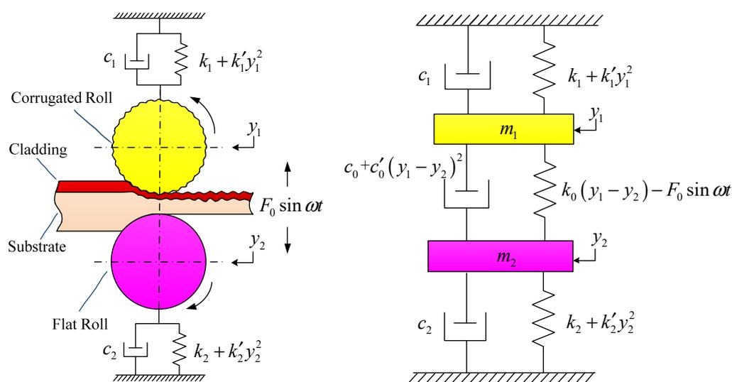
**Figure 1.** The rolling diagram of corrugated rolling mill: (left) the mechanical model; (right) two-degree-of-freedom vertical nonlinear vibration model.
