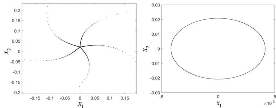
**Figure 6.** The stable periodic motion in 1:5 resonance when  $\mu = -0.01$ : (left) the stable fixed point; (right) the stable periodic motion.
