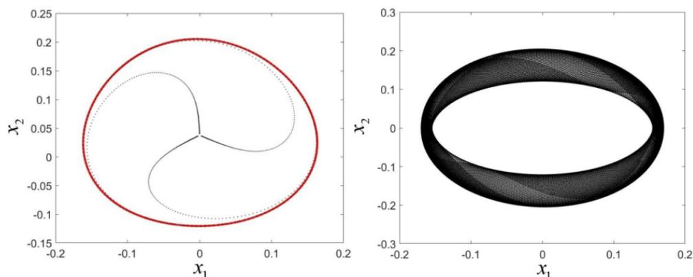
**Figure 3.** The stable quasi-periodic motion in 1:3 resonance when  $\mu = 0.01$ : **(left)** the stable invariant circle; **(right)** the stable quasi-periodic motion.
