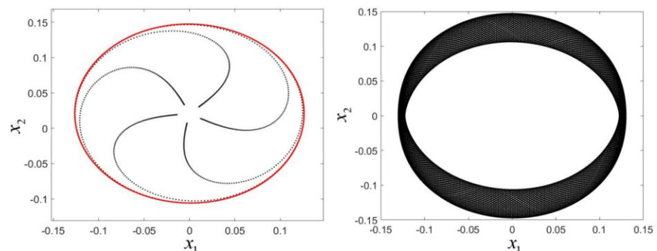
**Figure 7.** The stable quasi-periodic motion in 1:5 resonance when  $\mu = 0.01$ : (left) the stable invariant circle; (right) the stable quasi-periodic motion.
