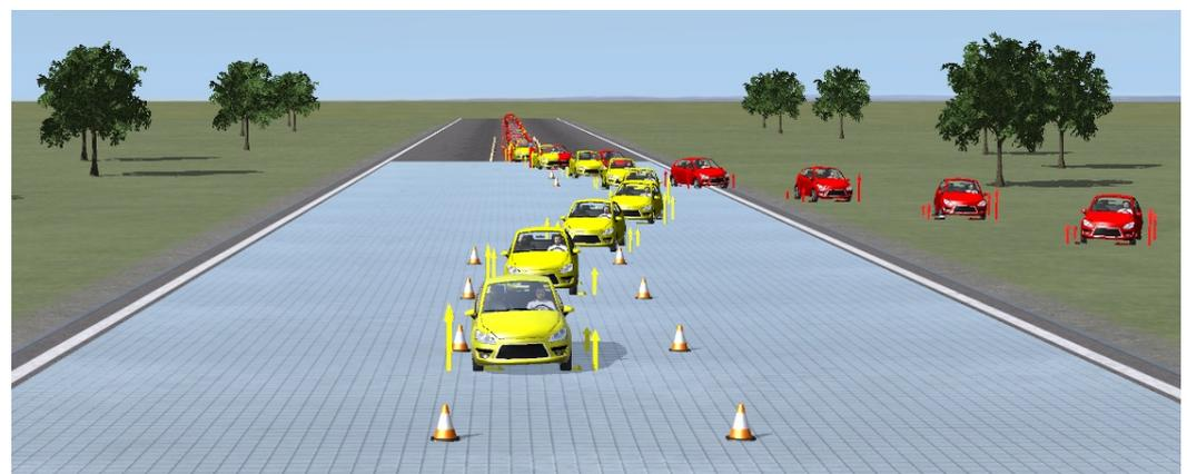
Figure 8. CarSim<sup>®</sup> DLC maneuver: open-loop vehicle (red), closed-loop vehicle (yellow).
