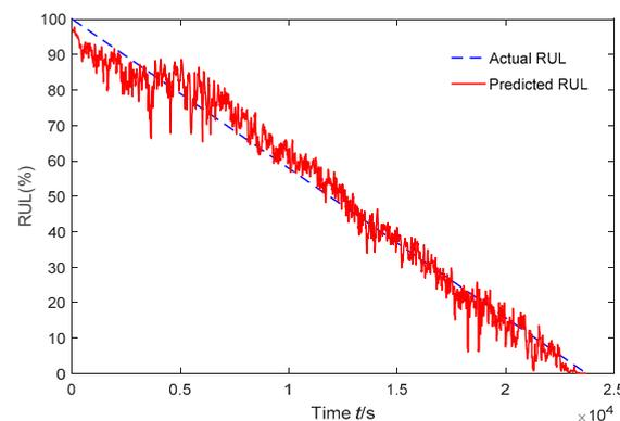
Figure 12. RUL prediction result of bearing 1\_3 using the proposed method.
