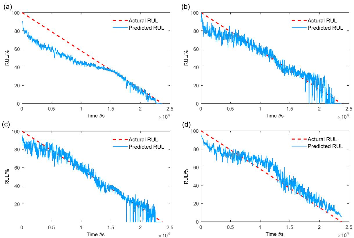
Figure 13. RUL prediction results of bearing1\_3 for four prognostics approaches: (a) ResNets; (b) CLSTM; (c) MS-DCNN; and (d) MS-DRN.
