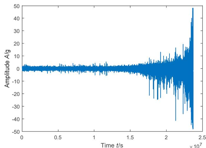
**Figure 9.** Whole life-cycle time domain waveform of bearing 1\_3.
