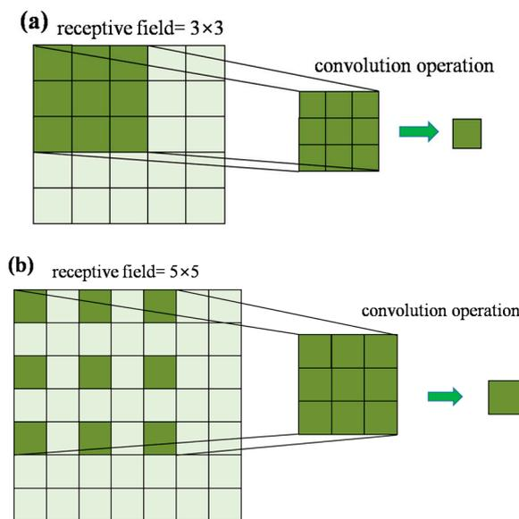
Figure 2. Convolution operation with different dilation factors: (a)  $d = 1$  and (b)  $d = 2$ .
