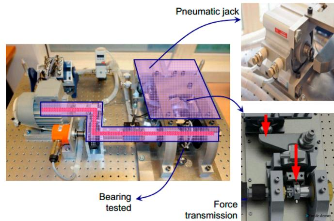
**Figure 8.** Bearing-accelerated degradation test rig.
