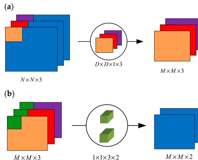
**Figure 4.** Depthwise separable convolution: (a) DWConv and (b) PWConv.
