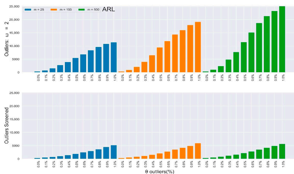
Figure 4. In-control ARL values of the multivariate Shewhart chart from a mixed distribution with and without SDRE multivariate outliers screening ( \omega = 2 ).
