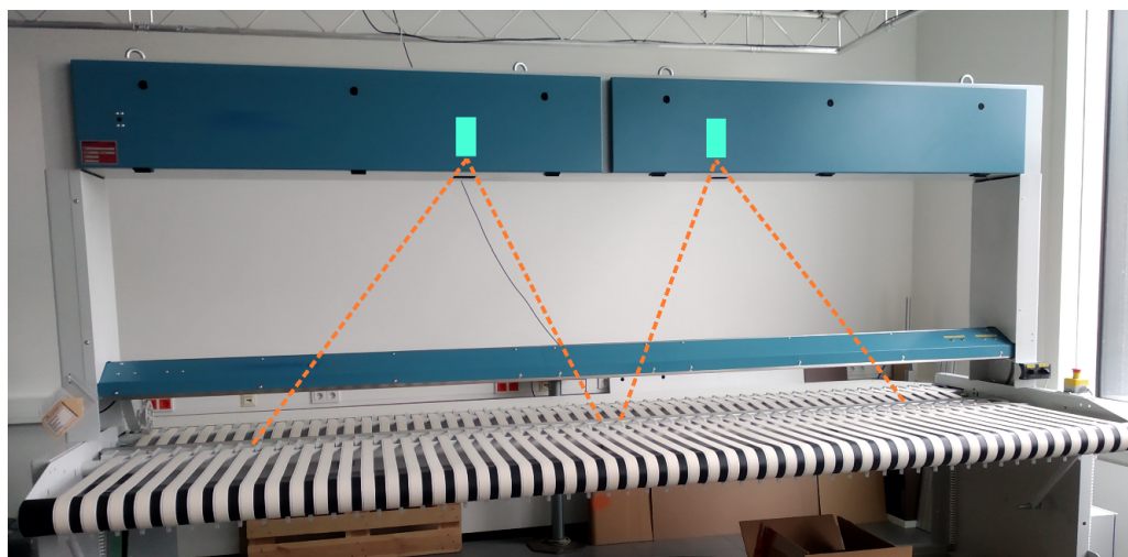
Figure 1. A photo of the image acquisition apparatus. The cyan rectangles show the positions of the line scan cameras. The dotted orange lines illustrate the field of view of each camera.
