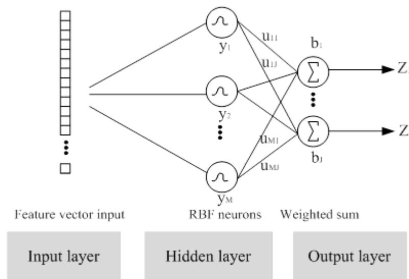
Figure 3. Typical architecture of an RBF neural network.
