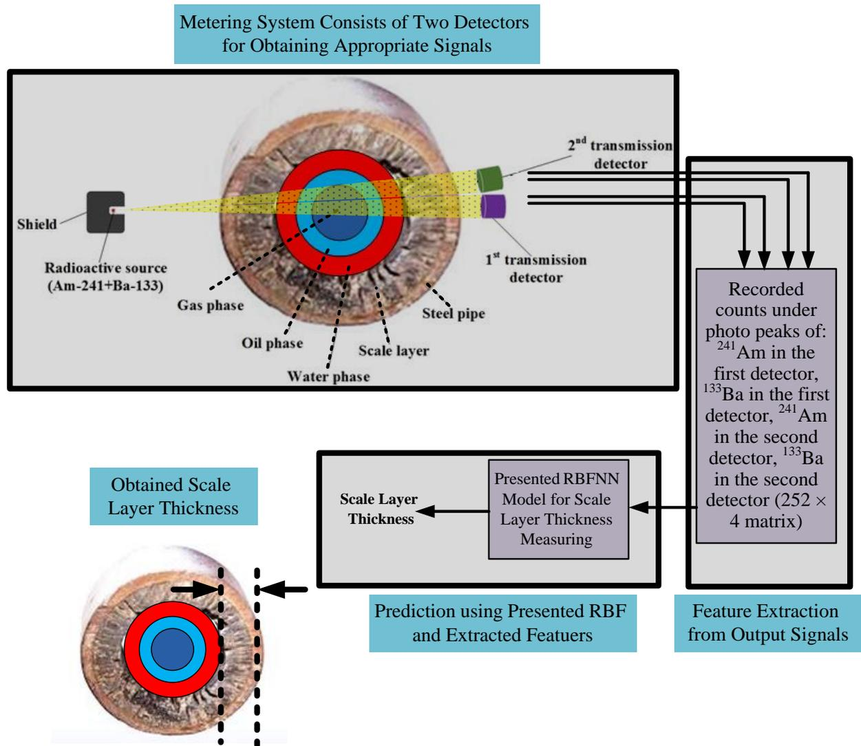
Figure 4. The conceptual procedure for scale layer thickness metering.
