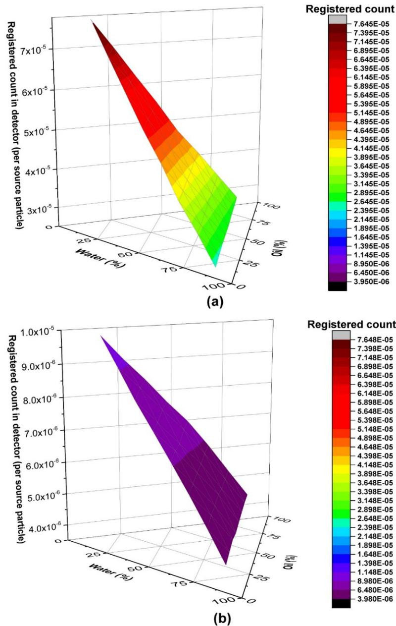
**Figure 6.** Recorded counts under the photopeak for the  $^{133}\text{Ba}$  radioisotope in the 1st detector for various combinations of volume fractions when the scale thickness is: (a) 0 cm, (b) 2 cm.
