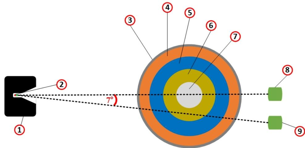
**Figure 1.** Simulated geometry: (1) Radiation shield, (2) Radioactive sources, (3) Steel pipe, (4) Scale layer, (5) Water phase, (6) Oil phase, (7) Gas phase, (8) First transmission detector, (9) Second transmission detector.
