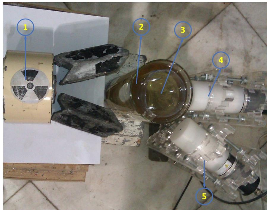
**Figure 2.** Experimental setup: (1) Radioisotope source, (2) Oil phase, (3) Gas phase, (4) 1st detector, (5) 2nd detector [20].
