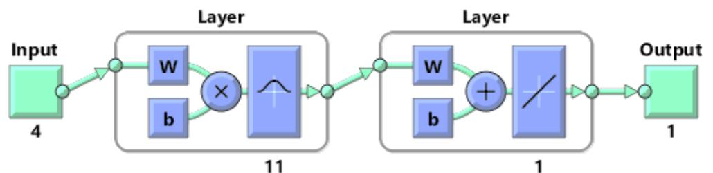
Figure 5. Schematic for the optimized RBF neural network.
