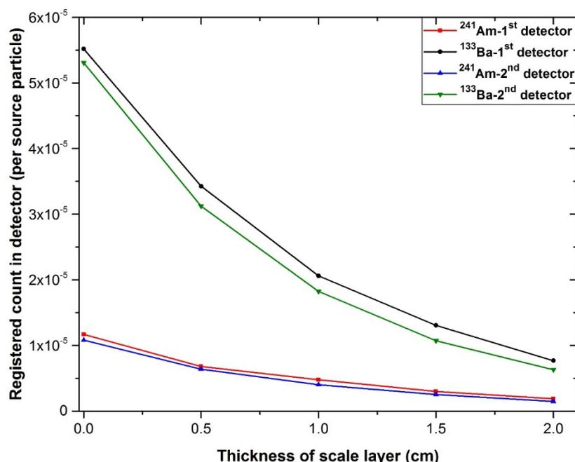
Figure 7. Registered counts in both detectors versus the changes in scale thickness for the state in which the volume fractions of components are fixed (50% gas, 30% oil, and 20% water).
