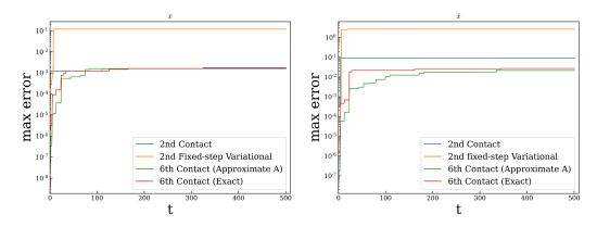
**Figure 12.** Maximum absolute errors in x and  $\dot{x}$  up to a given time for the reference contact integrators compared to the LSODA method along the orbit in Figure 11.
