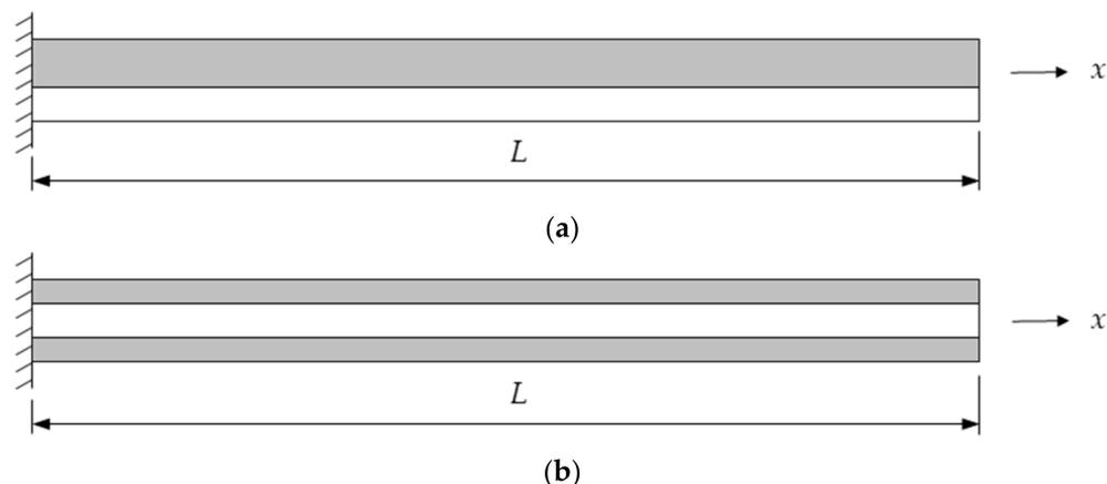
**Figure 1.** Elastic (□) and viscoelastic (■) material distribution in both FLD configurations: (a) Asymmetrical configuration; (b) Symmetrical configuration.
