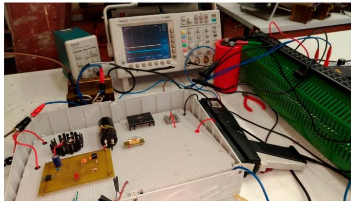
**Figure 3.** PWM controlled dc-dc boost converter prototype.
