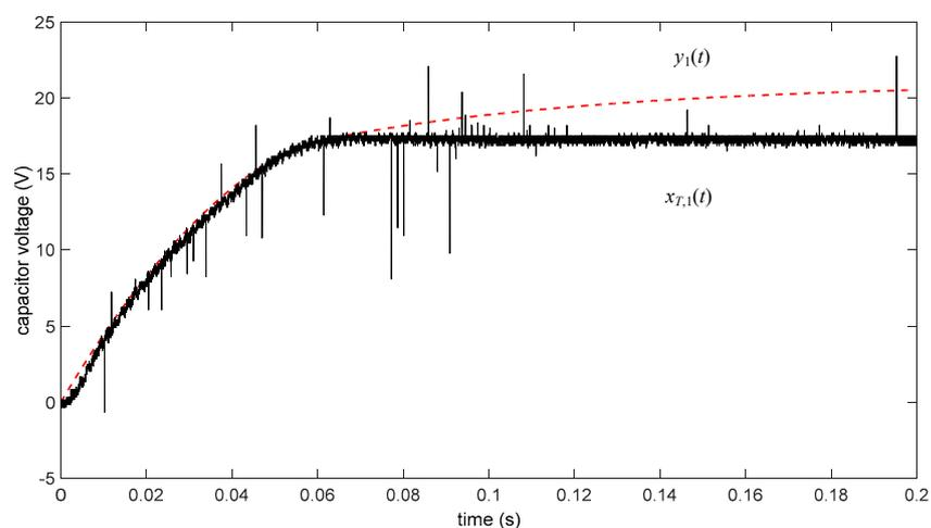
**Figure 5.** Transient of the voltage component  $x_1(t)$  of  $x_T$  and  $y_1(t)$  of  $y(t)$  for  $T = 1.52 \text{ ms}$ .
