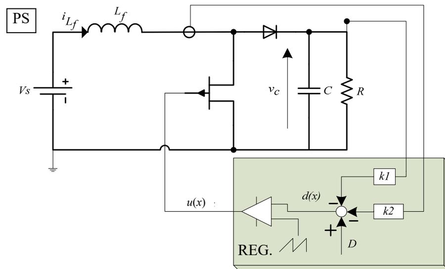
Figure 1. Circuital schema of a PWM controlled boost converter.
