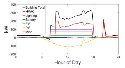
**Figure 2.** Power consumption profiles for the building and the individual subsystems under rules-based control scheme over a 24 h period.
