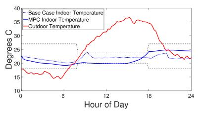
**Figure 8.** Indoor building temperature profiles under the rules-based control scheme and under the supervisory Peak Demand MPC with perfect forecasting, with upper and lower indoor temperature bounds (dashed black line), referenced with the ambient outdoor temperature.
