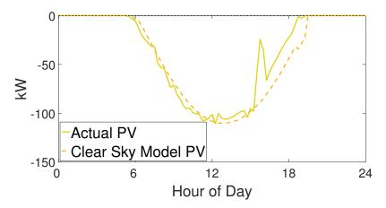
**Figure 5.** A comparison between actual photovoltaic (PV) power availability (solid line) and the power predicted by the clear sky model (dashed line) for a simulated day with high solar irradiance (29 June 2015).
