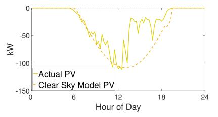
**Figure 6.** A comparison between actual PV power availability (solid line) and the power predicted by the clear sky model (dashed line) for a simulated day with low solar irradiance (1 July 2015).
