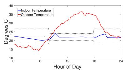
Figure 3. Time profiles of the building's indoor and outdoor temperatures under the rules-based control scheme.
