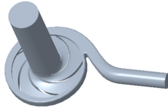
Figure 2. Computational flow domain of the investigated pump.
