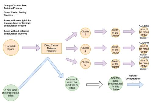
Figure 3. Work flow of the proposed method.
