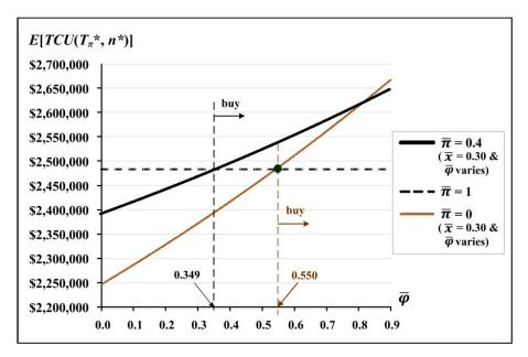
**Figure 12.** Impact of changes in  $\overline{\varphi}$  on  $E[TCU(T_{\pi}^*, n^*)]$  for managerial decision makings.
