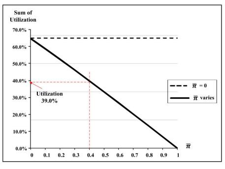
**Figure 10.** Impact of differences in  $\overline{\pi}$  on overall machine utilization.
