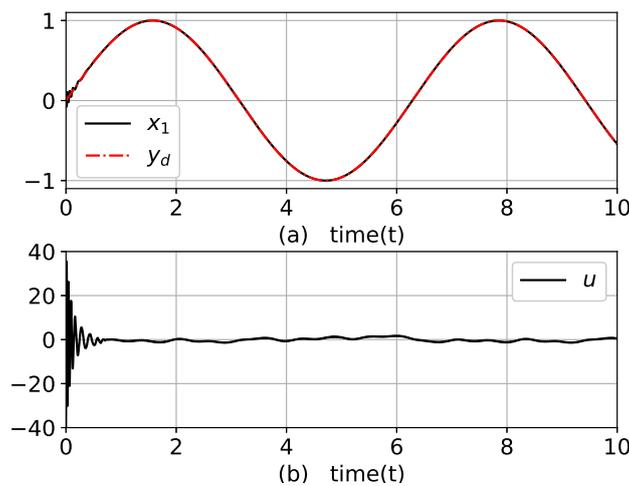
Figure 1. Trajectories of (a)  $y$  and  $y_d$  (b) control input  $u$  with  $\mathbf{x}(0) = [0.1, 0]^T$ .
