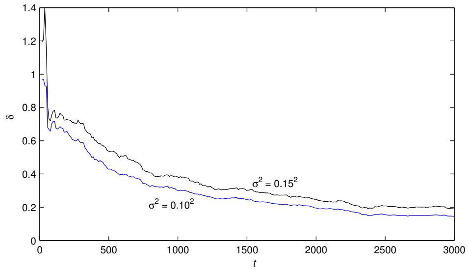
**Figure 2.** The RGLS parameter estimation errors  $\delta$  versus  $t$  with different variances.
