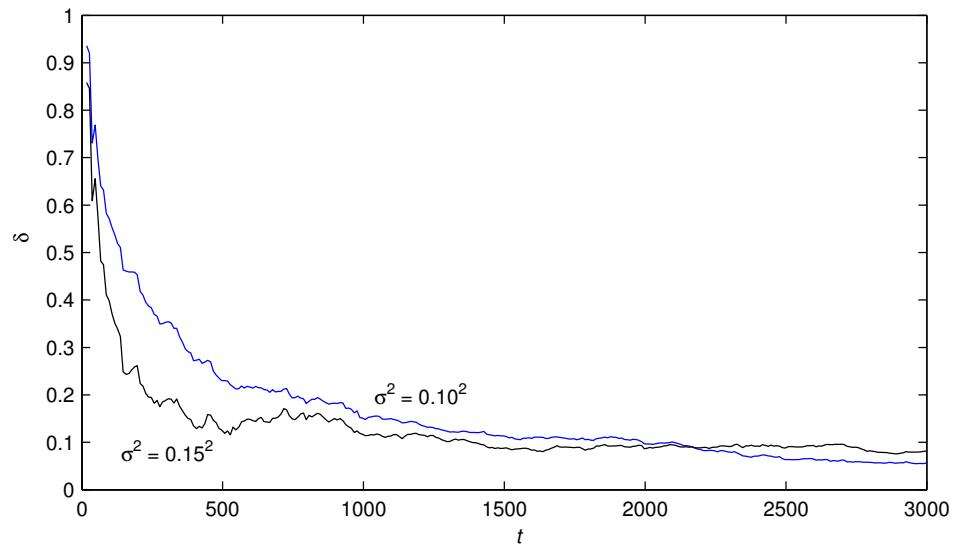
**Figure 3.** The F-TS-RGLS parameter estimation errors versus  $t$  with different variances.
