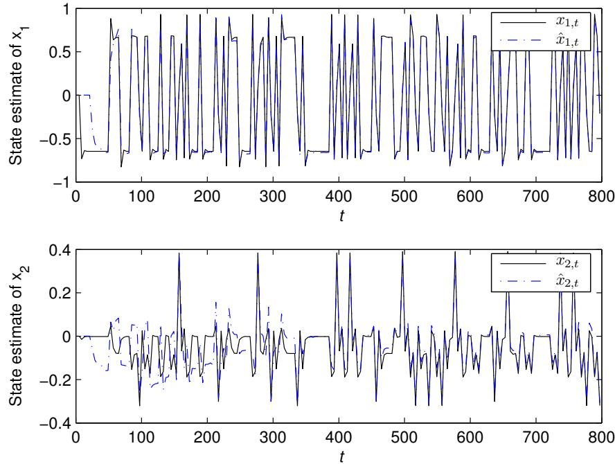
**Figure 6.** State  $x_t$  and its estimate  $\hat{x}_t$  versus  $t$  ( $\sigma^2 = 0.10^2$ ).
