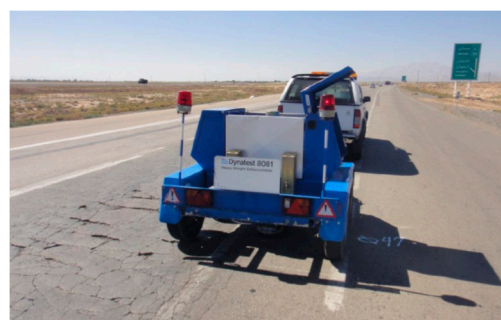
Figure 1. The heavy falling weight deflectometer (HWD) used in this study for determining the remaining service life (RSL).
