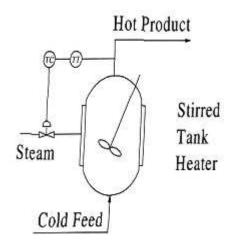
Figure 2. Stirred-tank heater.
