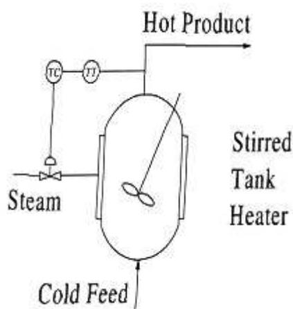
Figure 2. Stirred-tank heater.
