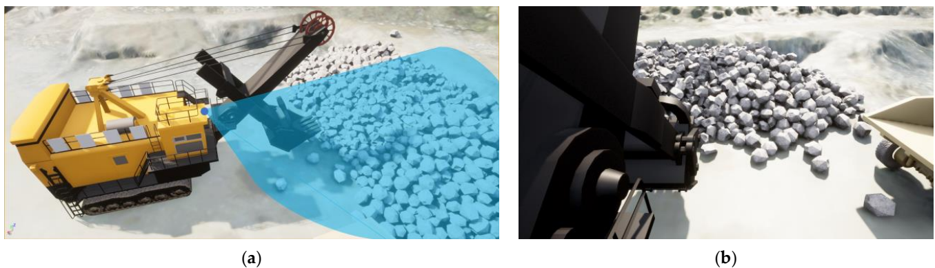
Figure 2. Sensor configuration in the Carla simulation. (a) Sensor mounting positions, where the blue region indicates the camera field of view. (b) Camera viewing direction.
