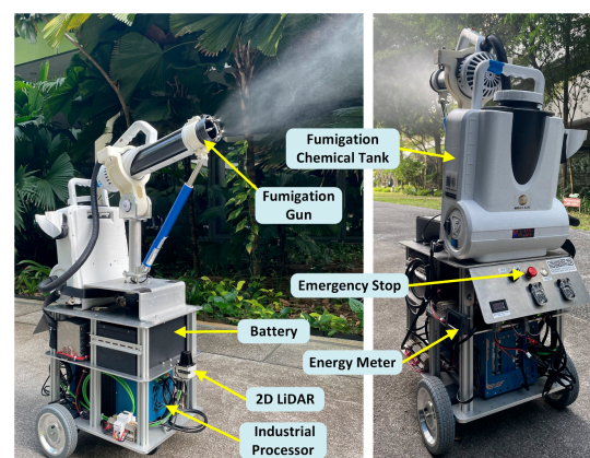
Figure 8. Developed autonomous fumigation robot.
