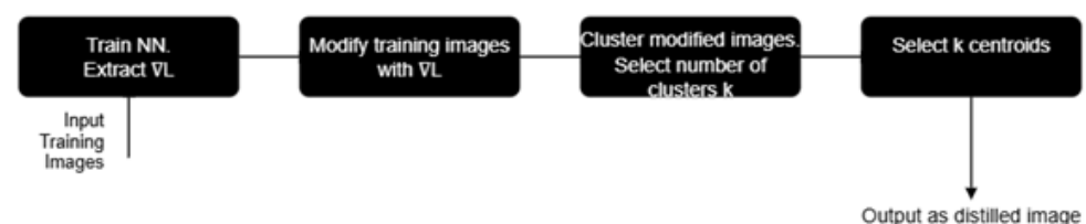
Figure 1. A flow chart describing the new distillation method. \nabla L denotes the gradient of the loss function; the clustering is class-wise.
