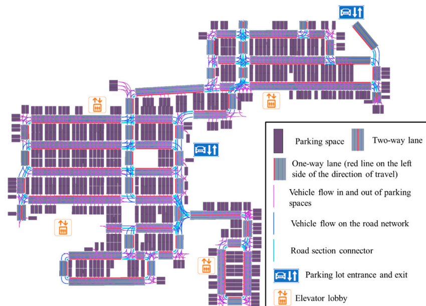
Figure 5. Parking Lot Internal Structure.
