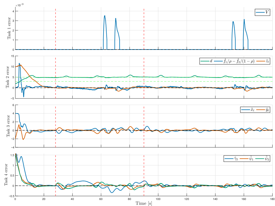
Figure 9. Formation control errors occur when the system is disturbed by a wind of approximately 20 km/h in the positive x -axis direction.
