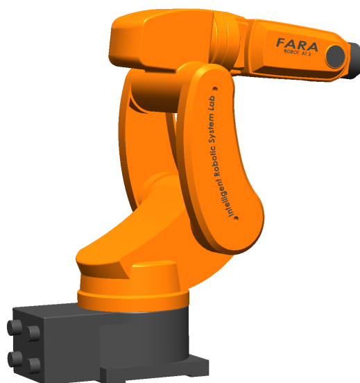
Figure 3. Three-dimensional SolidWorks model of the Samsung FARA AT2 robotic arm.
