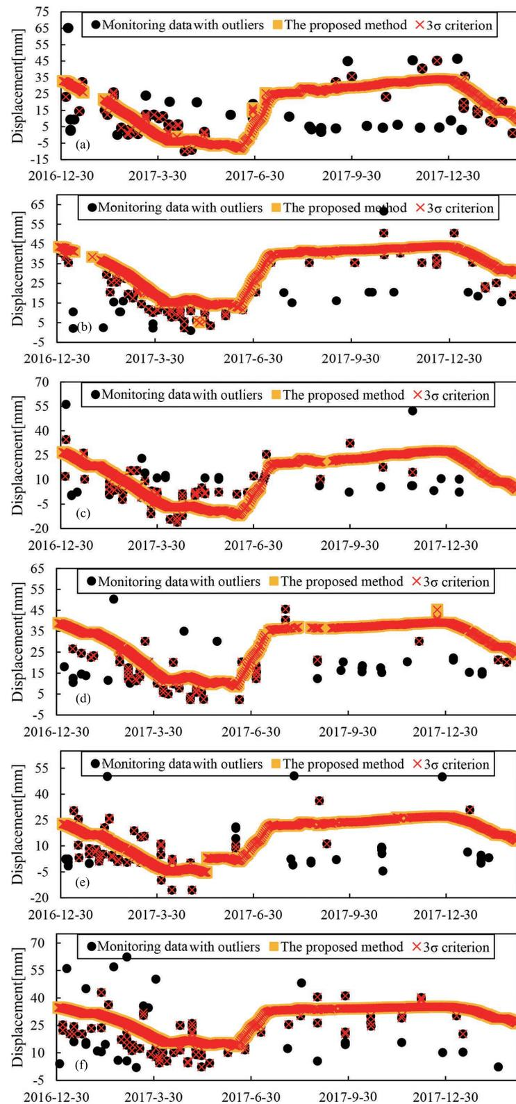
**Figure 11.** The results of outlier detection of the proposed method and  $3\sigma$  method of: (a) PL11-1, (b) PL11-3, (c) PL13-1, (d) PL13-3, (e) PL16-1, and (f) PL16-3.
