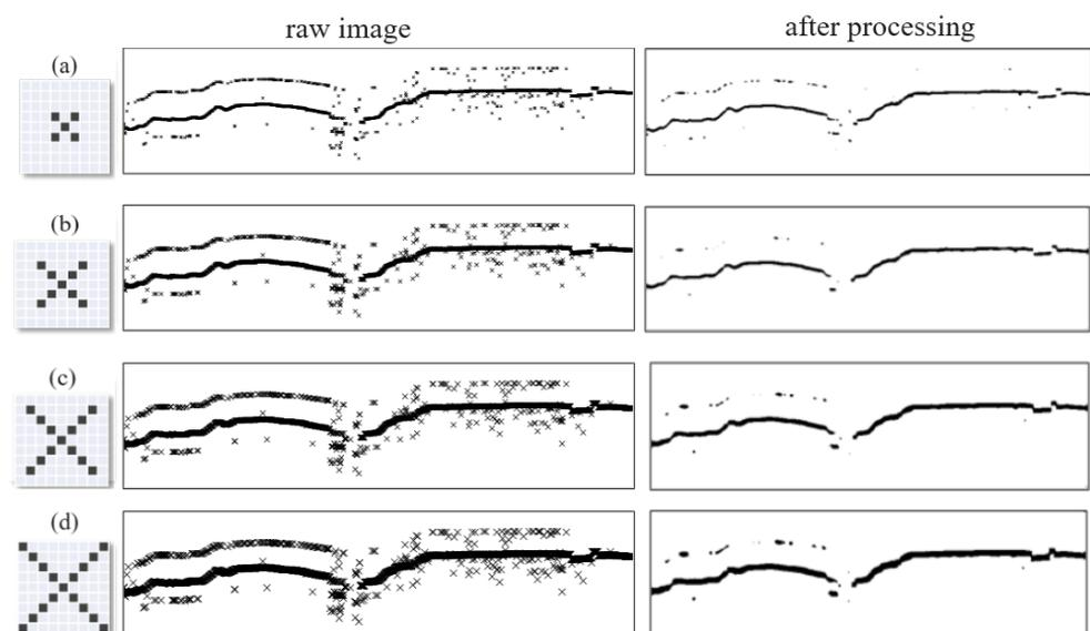
**Figure 9.** Gaussian blur and Ostu binarization processing scatter plots using a cross with different sizes: (a) 5 pixels, (b) 9 pixels, (c) 13 pixels, and (d) 17 pixels.
