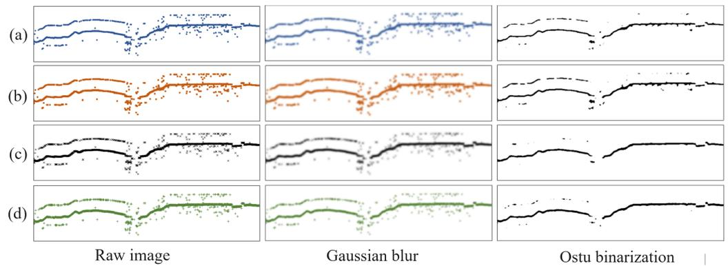
**Figure 8.** Gaussian blur and Ostu binarization of a plot using different shapes of scatters: (a) circle, (b) square, (c) cross, (d) isscross.
