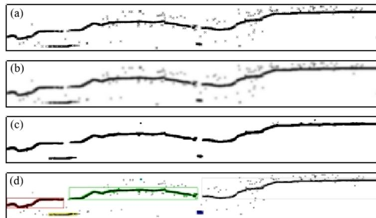
**Figure 10.** The error processing of the sample data sequence using the proposed method: (a) raw image, (b) Gaussian blur, (c) Ostu binarization, and (d) process line identification.
