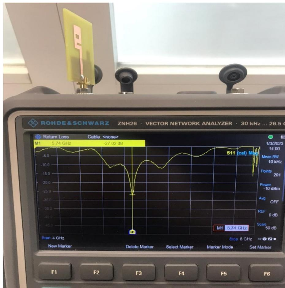
**Figure 5.** Return loss measurement of an e-shaped antenna using VNA.
