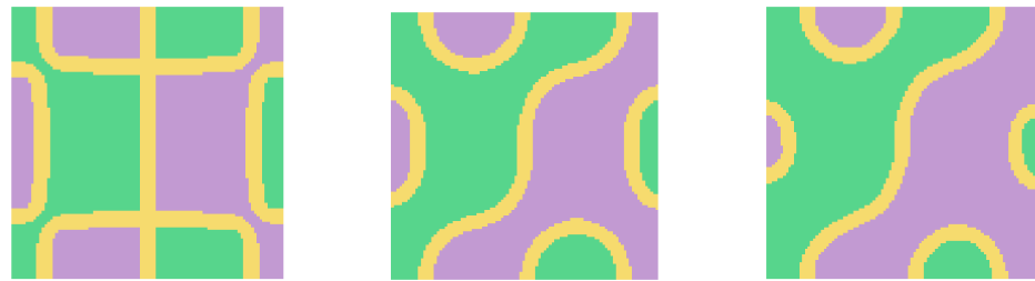
Figure 9. Electrode profile for the 7th mode. Without volume constraints (left), V = 0.20 (center) and V = 0.15 (right).
