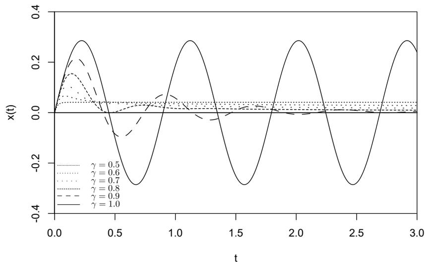
**Figure 3.** Free undamped fractional harmonic oscillator in (14) for  $t \in [0, 3]$ ,  $b_1 = 2$ , and  $\omega_0 = 7$ .
