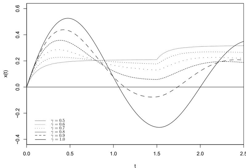
**Figure 2.** The solution of the fractional harmonic oscillator with constant forcing, as given in (13), evaluated for  $t \in [0, 2.5]$ ,  $A = 1$ ,  $B = 1$ ,  $b_1 = 2$ ,  $c = 1.5$ , and  $\omega_0 = 3$ .
