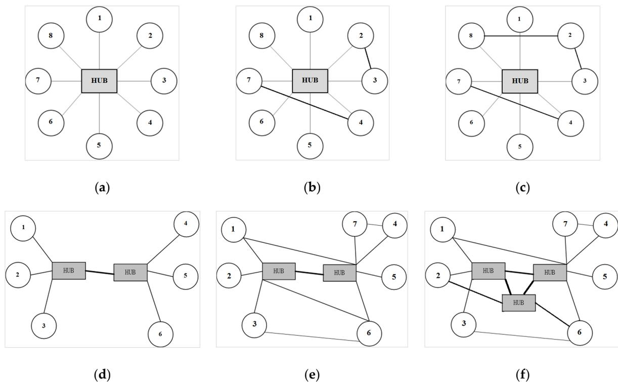
**Figure 1.** Sample *H-S* network typologies. (a) Single-hub location and allocation; (b) single-hub location and allocation with *N-N* links; (c) single-hub location with *N-N* links; (d) two-hub location and single-allocation; (e) two-hub location and multi-allocation with *N-N* links; (f) multi-hub location and multi-allocation with *N-N* links.
