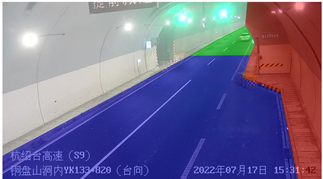
**Figure 10.** Highway tunnel for C005. Blue and green represent the high-speed incoming and outgoing flows in Figure 9b, respectively, while red and white represent the filtering area (static traffic signs and strong light false detection).
