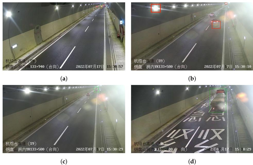
**Figure 2.** Illustration of challenges in MCMVT for highways. (a) represents the target scale variation, in which the yellow, orange and red bboxes respectively represent no occlusion at high scores, slight occlusion at high scores and severe occlusion at low scores; (b,d) represents intense lighting in the tunnel; (c) illustrates vehicles within green boxes being captured by adjacent cameras at the same time.
