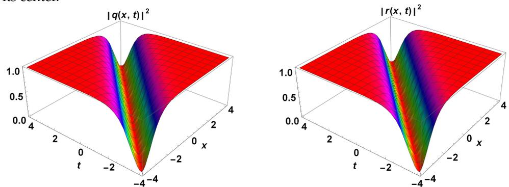
**Figure 2.** Profiles of a dark 1-soliton along the two components of a birefringent fiber after neglecting the radiative effects.
