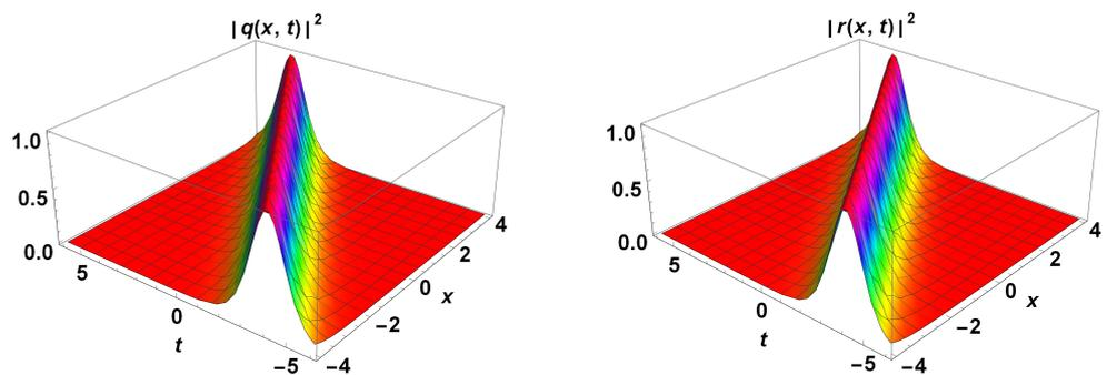
Figure 1. Profiles of a bright 1-soliton along the two components of a birefringent fiber after neglecting the radiative effects.
